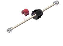
5. Slide the GM67X-CS-R or GM67X-CS-B seal nut onto GM67X-CS-R or GM67X-CS-B body as shown then screw down seal nut enough to allow it to remain on body but not enough to restrict motion of GM67X-CS-R or GM67X-CS-B assembly.
